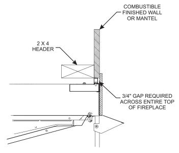
Figure 7 - Clearances to Combustibles
