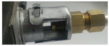
Figure 3 - Air Shutter Fully Open
