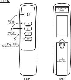
This remote control Transmitter allows the user to turn the fireplace on and off, and adjust the flame height.
