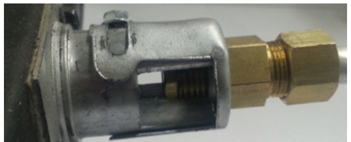
Figure 3 - Air Shutter Fully Open
