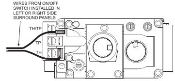
NOTE: TO OPERATE INSERT WITH SIDE PANEL ON/OFF SWITCH, BE SURE TO PLACE THE MAIN SWITCH (TO THE RIGHT SIDE OF GAS VALVE) TO "OFF" POSITION
