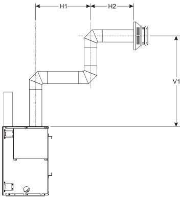
If total horizontal needs to be 10' (3.05 m), then the minimum required vertical is 7' (2.13 m).
