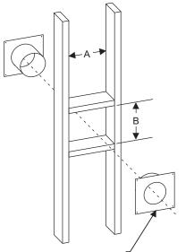
WALL FIRESTOP HOLE IS OFF-SET TOWARDS BOTTOM OF WALL OPENING
