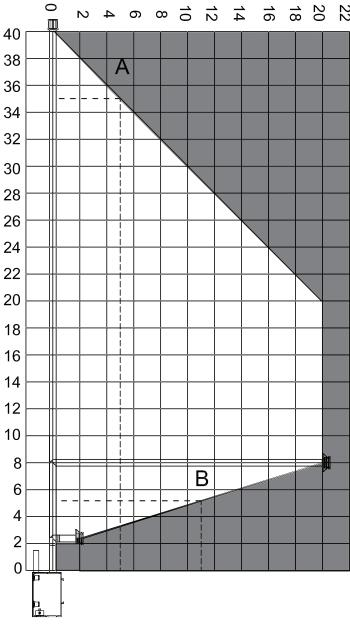
Acceptable vertical and horizontal vent run. (40 ft. (12.19 m) maximum vertical and 20 ft. (6.10 m) maximum horizontal)
