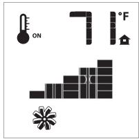
Figure 31 - Fan Speed Control Activated
