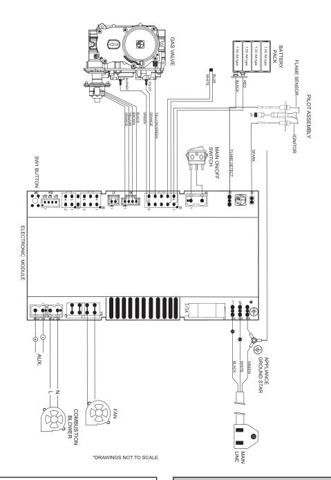
If any of the original wire as supplied with this unit must be replaced, it must be replaced with equivalent gauge and temperature rated wire.
