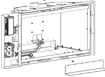
17. Pull blower far enough through the blower access hole to disconnect the wires at the connectors. **See Figure 43.** Once the wires are disconnected, remove blower completely and discard.
