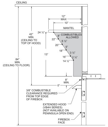
Figure 3b - Mantel Clearances with Optional Extended Hood
