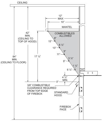
Figure 3a - Mantel Clearances with Standard Hood
