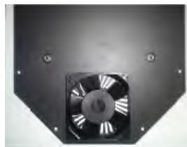
Fan on Access Panel
