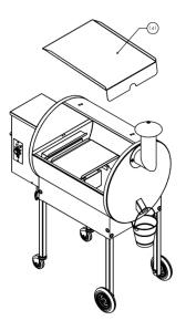
**RECOMMENDATION** for ease of clean-up: Line the Grease Drain Pan (141) with Heavy duty aluminum foil. Be sure the edges and ends of the foil are tight against the bottom of the Grease Drain Pan (141).
