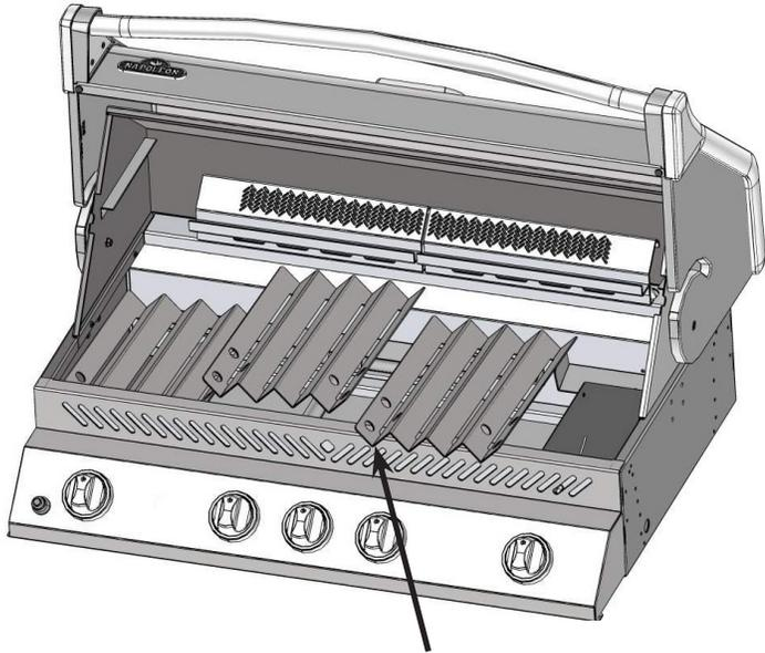
*Ensure holes in sear plates are positioned to the front of the grill.*
