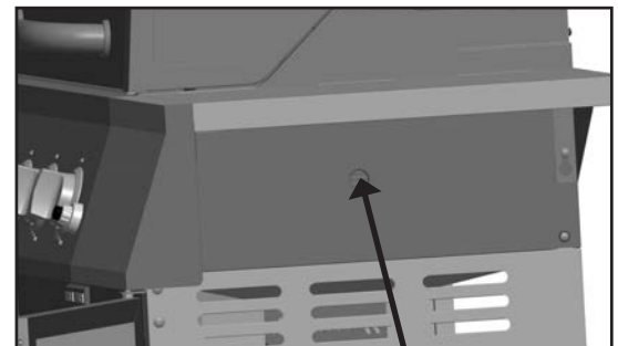
Hole for viewing the flame
