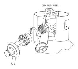
7) Open tank valve fully (counterclockwise). Use a soapy water solution to check all connections for leaks before attempting to light grill. If a leak is found, turn tank valve off and do not use grill until a local L.P gas dealer can make repairs.
