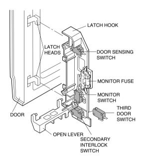
Figure C-1. Latch Switch Adjustments
