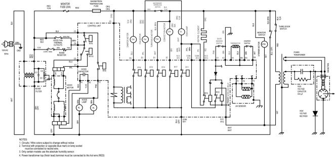
Figure O-1. Oven Schematic - Off Condition
