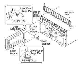
Figure C-2. Door Replacement and adjustment
