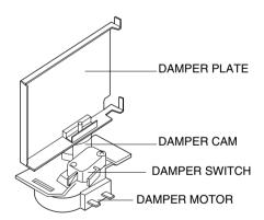
Figure D-2. Damper Mechanism
