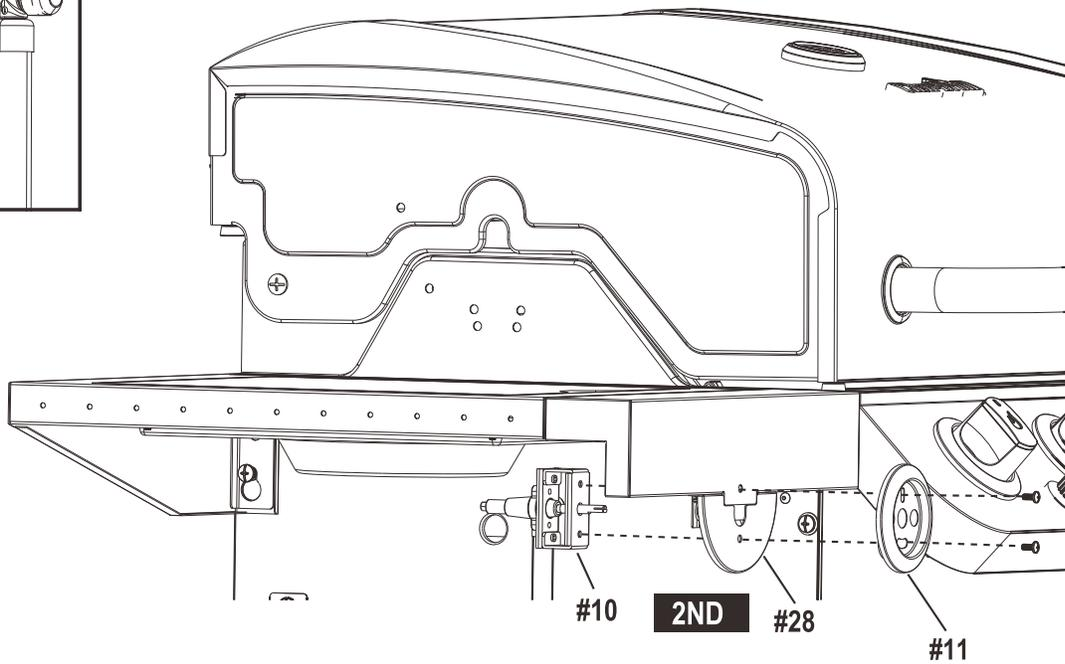
Secure using screws that were removed from sideburner valve bracket.
