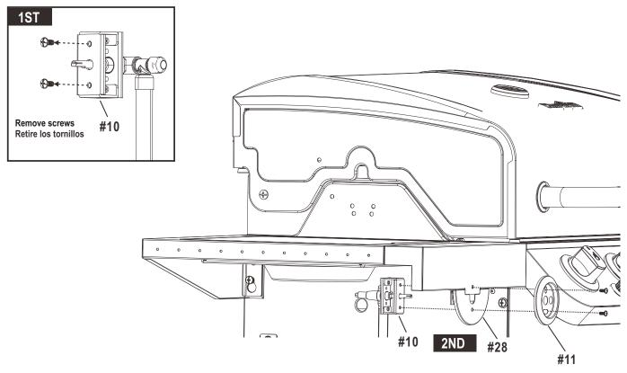
Secure using screws that were removed from sideburner valve bracket. Fíjelo con los tornillos que retiró del soporte de la válvula del quemador lateral.
