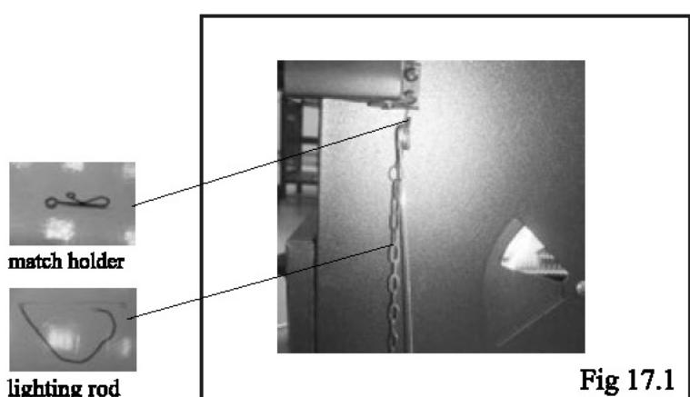
3. Use the match holder to secure and direct the match into the hole to burner, when igniter is not working. Fig 18.1
