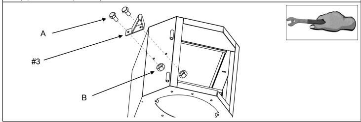
Step 14. Assemble Firebox Lid (Part #4) using 1 pc of Bolt M5 x 10 (I) and 1 pc of Washer M6 (H) on Firebox (Part #5)
