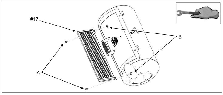
Step 8. Assemble Front Table Brackets (Part# 18) using 2 pcs of Bolt M6 x 14 (C) on Front Table (Part # 17). Then use 2 pcs of Bolt M8 x 16 (A) and 2 pcs of Nut M8 (B) to assemble on Main Chamber Body (Part# 2)
