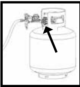
Apply solution to gas cylinder valve.
