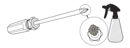
Tools Required for Assembly and Leak Testing (not included): Phillips screwdriver, Spray bottle
