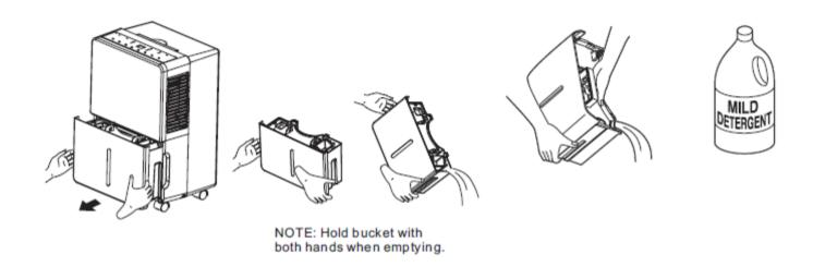
NOTE: When the bucket is full or removed from the machine, the compressor will turn off, but the fan will continue to run for a few minutes. This is completely normal. The dehumidifier will not be removing moisture from the air at this time.
