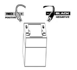
REMOVE TIMER KIT COVER AND INSTALL A 6 V RECHARGEABLE BATTERY (NOT INCLUDED) BY ATTACHING RED ALLIGATOR CLIP TO THE POSITIVE TERMINAL (+) AND BLACK ALLIGATOR CLIP TO THE NEGATIVE (-) TERMINAL.
