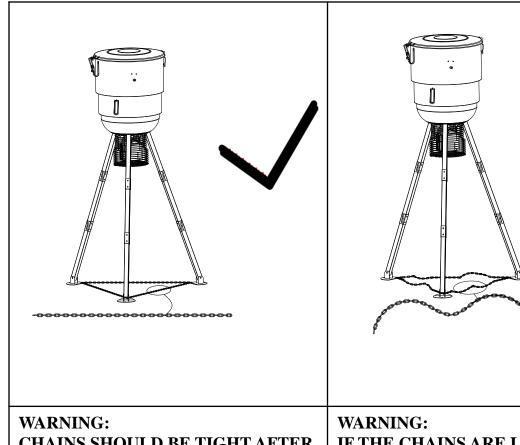
CHAINS SHOULD BE TIGHT AFTER ASSEMBLY. IF CHAINS ARE TIGHT THEN YOUR FEEDER IS ASSEMBLED CORRECTLY AND SAFELY. IF THE CHAINS ARE LOOSE OR MISSING AFTER ASSEMBLY, THEN YOUR FEEDER IS ASSEMBLED INCORRECTLY. IT IS EXTREMELY UNSAFE AND WILL POTENTIALLY FALL DURING USE RESULTING IN SERIOUS INJURY OR DEATH.
