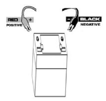
REMOVE TIMER KIT COVER AND INSTALL A 6V RECHARGEABLE BATTERY (NOT INCLUDED) BY ATTACHING RED ALLIGATOR CLIP TO THE POSITIVE TERMINAL (+) AND BLACK ALLIGATOR CLIP TO THE NEGATIVE (-) TERMINAL.
