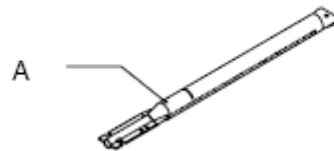
A. Air shutter adjustment screw
