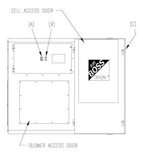
Control Switch (A): The control switch is located on the cell access door. It controls the operation of the
