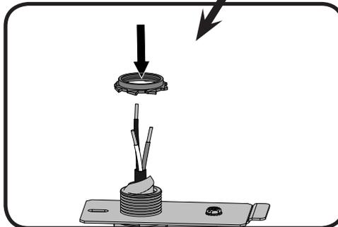
Connect the ground green wire to the junction plate using the grounding screw (W570-0098). Using the wire connectors, connect the common white wires together, then the hot black wires.
