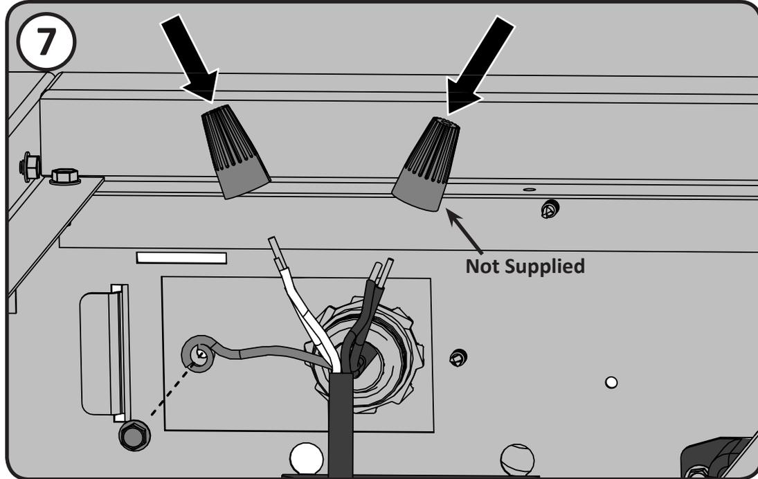
Reinstall the electrical box as shown.
