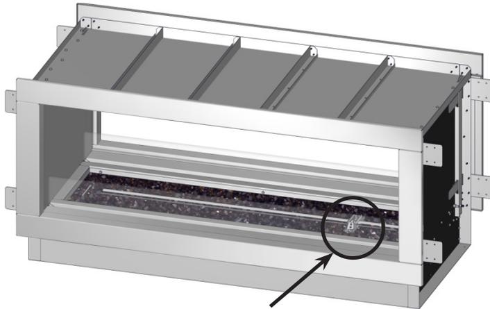
ENSURE NO GLASS IS PLACED ON THE IGNITION PORTION OF THE BURNER, DIFFICULTIES IN LIGHTING MAY RESULT.
