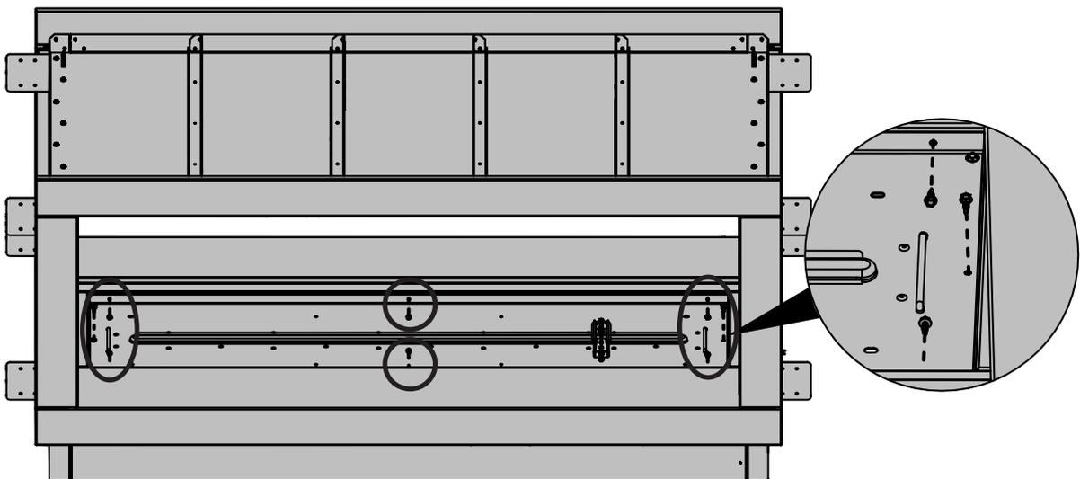
Lift the burner tray with the handles as illustrated.
