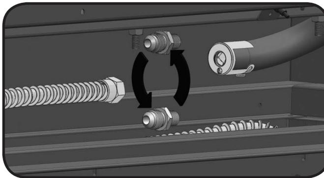
6. Replace the natural gas orifice with the LP (Propane) orifice supplied. Note: The air shutter has been factory set and does not need to be adjusted.
