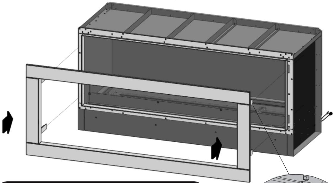
**!** **NOTE!** If using facing materials in excess of 2.5" (63.5mm) a gap will be visible between the brick ledge and the trim.
