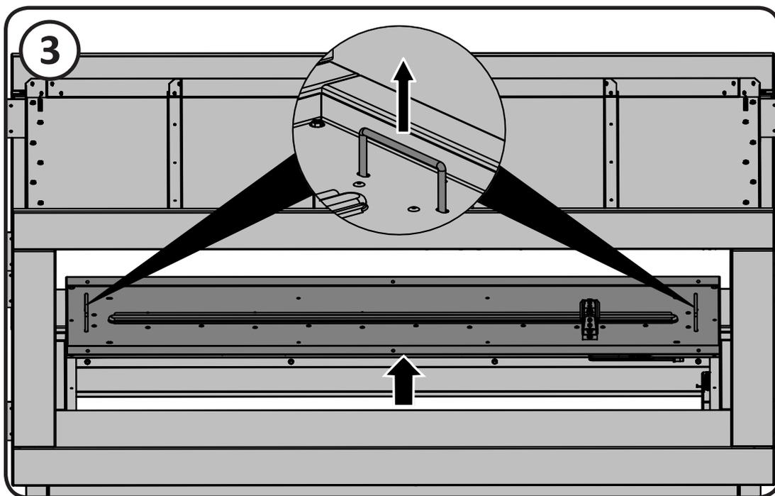
Remove the screw (N570-0008) from the electrical box cover.
