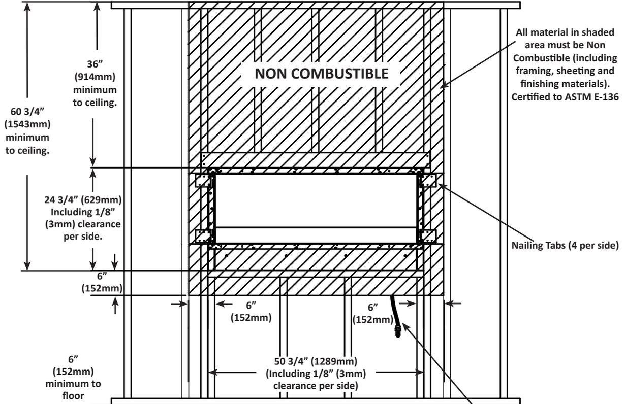
**NOTE!** Ensure top of cabinet is closed to prevent rain and debris from falling on top of the appliance.
