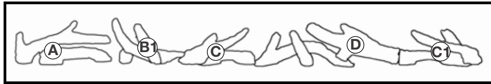
Recommended driftwood log placement for NEFL60CHD-1
