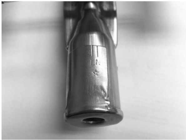
Burner Set at LP
