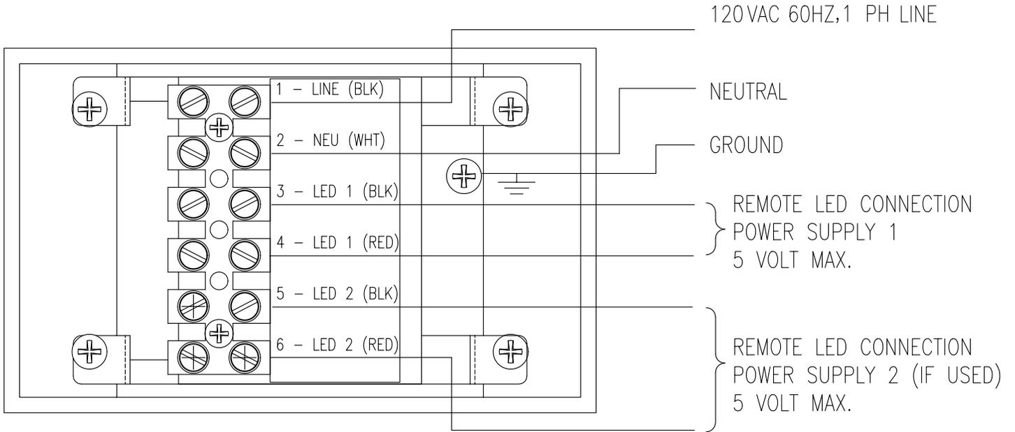
Figure 4 - Wiring Diagram KES-2
