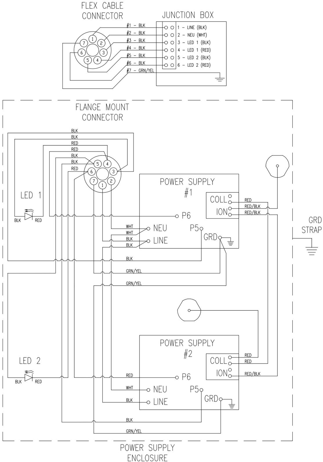
Figure 6 - Remote Mounted Control Box Schematic
