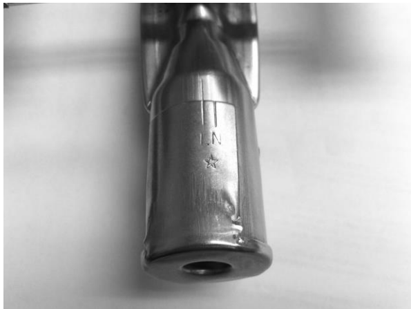
Burner Set at LP
