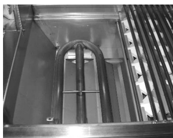
Grill U-Burner (Standard) located underneath the briquette trays.
