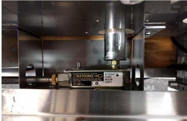
CORRECT INSTALLATION THE ORIFICE IS COMPLETELY INSERTED INSIDE THE VENTURI
