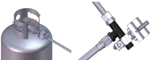
Propane tank: height = 456mm, diameter = 320mm
