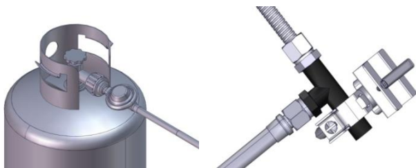
Propane tank: height = 456mm, diameter = 320mm
