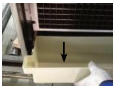
1-d. Take out the water box and empty out the water.
