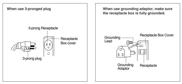
"THE CANADIAN ELECTRICAL CODE DOES NOT ALLOW THE USE OF THE GROUNDING ADAPTOR"
