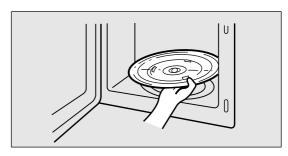
The roller guide and oven cavity floor should be cleaned regularly to avoid excessive noise.
