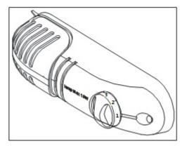
• Turning the temperature control knob to "0" position stops the cooling cycle but does not shut off the power to the unit.
