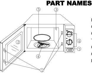
Door Safety Lock System Oven Window Oven Air Vent Turntable roller Glass Tray Control Panel Door Release Button
