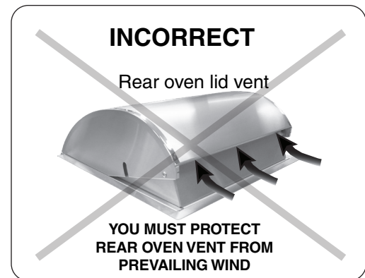
Fig. 8-3 Airflow direction - INCORRECT
