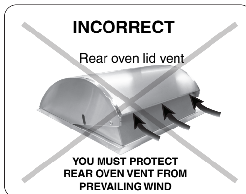
Fig. 8-3 Airflow direction - INCORRECT
