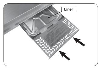
Fig. 24-1 Install drip tray
