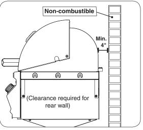
Fig. 9-1 Clearance 'A' Diagram
