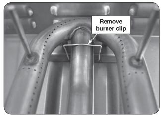
Fig. 33-1 Main burner removal
