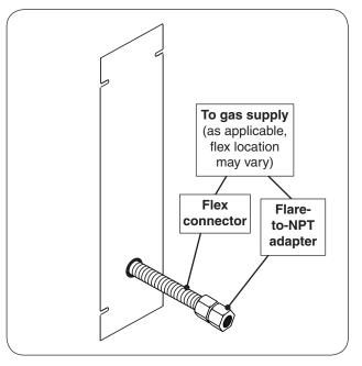
Fig. 18-1 Connect gas and secure plate
