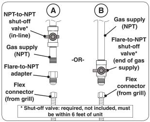
Fig. 18-2 Connecting to a gas line
