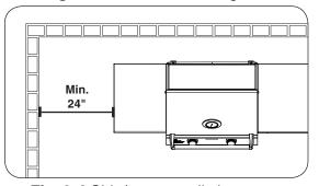
Fig. 9-4 Side/corner wall clearance
