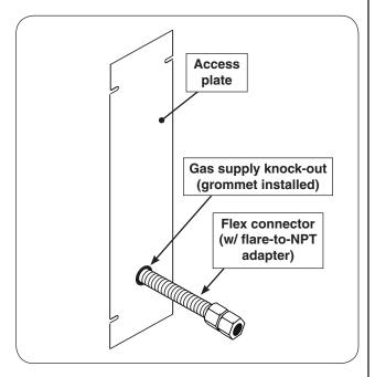
Fig. 17-1 Access plate view & install orientation
