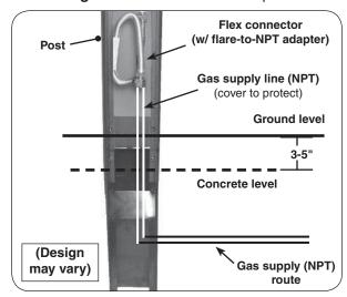
Fig. 20-3 Pour concrete & install post
