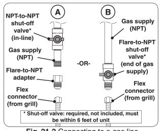
Fig. 21-2 Connecting to a gas line
