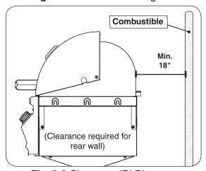
Fig. 9-3 Clearance 'B' Diagram
