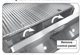
Fig. 22-4 Remove control panel
