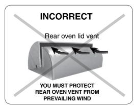
Fig. 10-3 Airflow direction - INCORRECT
