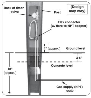
Fig. 19-1 In-ground install orientation
