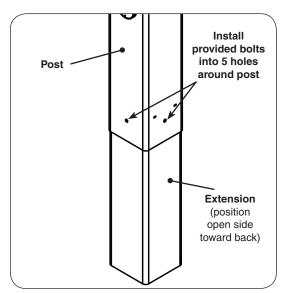
Fig. 20-1 Install extension to post
