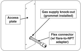
Fig. 20-4 Access plate view & install orientation
