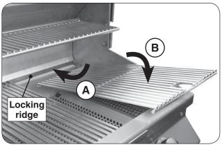
Fig. 22-2 Install cooking grids
