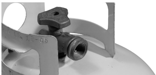
LP cylinder with type 1 valve connection
