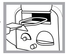
• Unplug starter and remove from ProZone™. Be careful when removing electric starter, the element will be very hot. After use, let element rest on support and cool completely away from children and pets.
