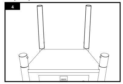
Insert Rear Side Shelf Brackets (with Supporting Pieces) into rear Side Posts. Make sure the supporting pieces are facing inward.
