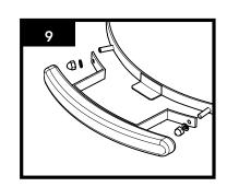
Close lid and press top vent onto top of Kamado so spring clips are fully engaged, with calibrations facing the front of the grill.
