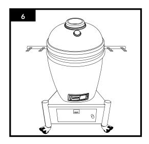
Place Fire Bowl back into the Grill with the bottom opening lining up with bottom draft door.
