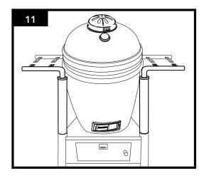
To attach Side Shelves remove the washers and the bolts from the bottom of the Shelves.
