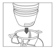
Take all parts out of the grill before lifting. With the help of a second person, lower the grill into the Stand by holding the back hinge and bottom of grill. As grill is lowered into stand, carefully switch out hands from bottom of grill to the ash drawer opening before reaching the outer ring of stand. Completely lower grill to bottom of stand.
