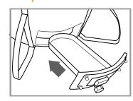
Slide Ash Drawer into ash drawer opening. When grill is cool, it is safe to remove ash from Ash Drawer. To remove Ash Drawer, use bottom knob on Ash Drawer, lift slightly and pull drawer out.
