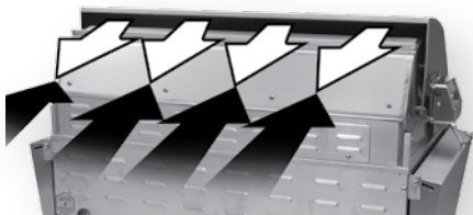
Wind hitting the back of the grill can disrupt proper exhaust.
