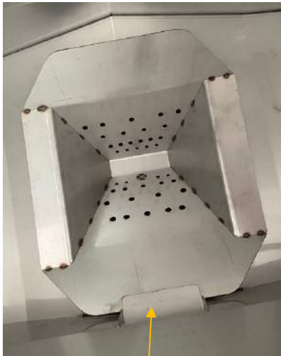
Correct Burner Pot Installation
