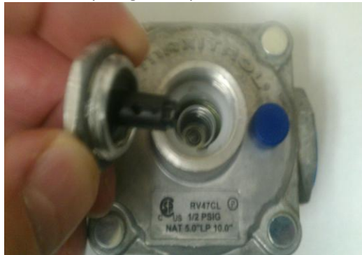
Regulator Converted to Natural Gas (NG)
