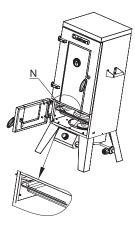
Step 11: Open bottom door and slide water/wood chip tray into built
