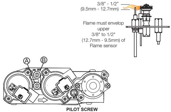
Prior to pilot adjustment, ensure that the pilot assembly has not been painted. If overspray or painting of the pilot assembly has occurred remove the paint from the pilot assembly, or replace. Fine emery cloth or a synthetic scrub pad (such as Scotch-Brite™) can be used to remove the paint from the pilot hood, electrode and flame sensor.
