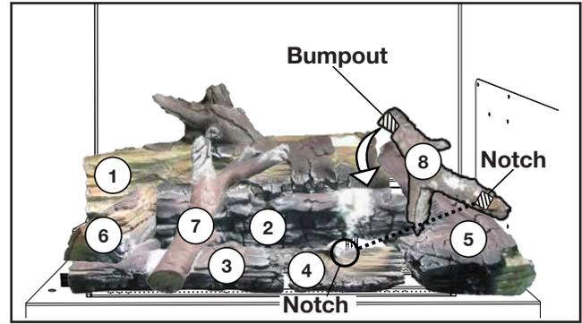
8. Hook the bumpout in log #8 around the back of log #7. Place the notch in log #8 on the notch in log #2.
