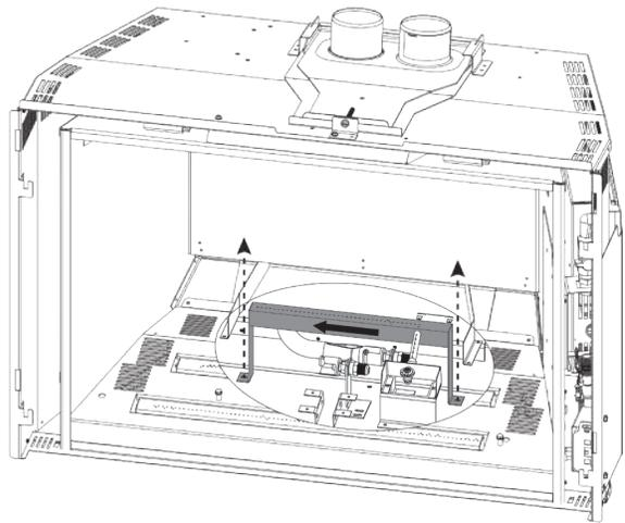
4. Remove the 2 screws securing the rear burner in place. Slide the rear burner to the left and out.
