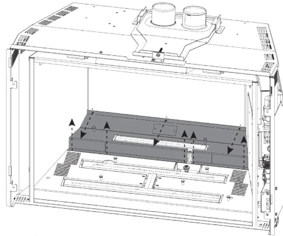
2. Remove the 8 screws securing the upper burner support in place. Lift the upper burner support up and out.
