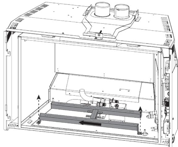
6. Remove the 2 screws securing the front burner in place. Slide the front burner to the left and out.
