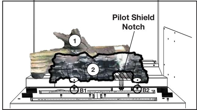
2. Place the two holes in log #2 on B1 and B2, ensuring the notch fits around the pilot shield.
