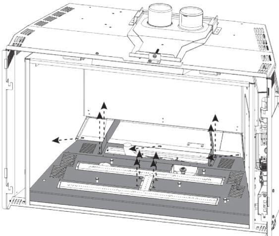
5. Remove the 7 screws securing the lower burner support in place. Remove the 4 screws securing the deflectors in place, and then remove the deflectors. Lift the lower burner support up and out.
