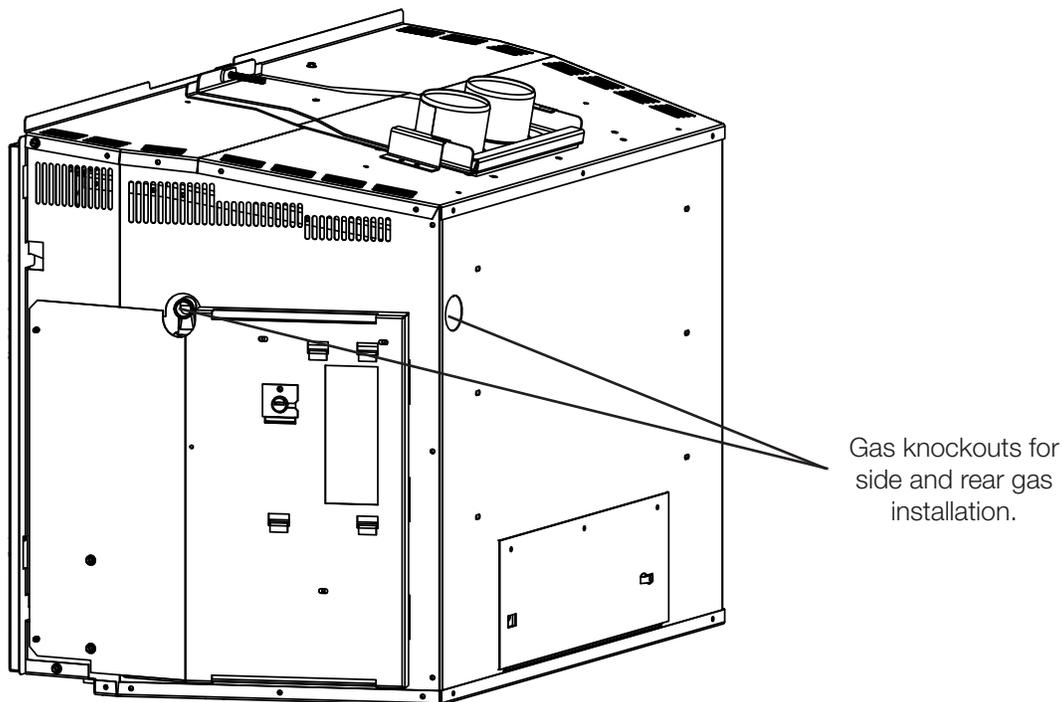
Gas knockouts for side and rear gas installation.
