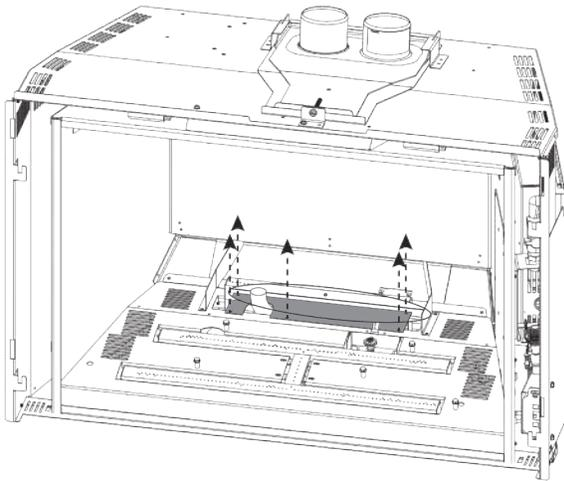
3. Remove the 5 screws securing the cover plate in place. Slide the cover plate back and out.
