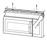
Remove the cover screw,pull the cover forward and then lift up the bulb holder.
