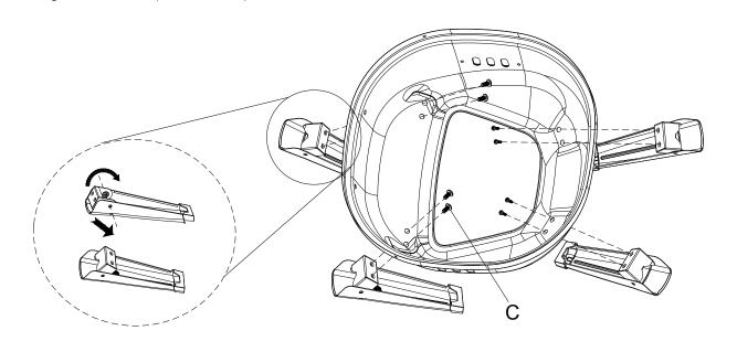
**Step 4**Attach bottom air damper to bottom bowl (B Screw 4Pcs / D Wing nut 4Pcs).
